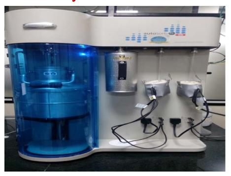
**BET Surface Area Analyzer:** Quanta chrome Autosorb iQ2 BET Surface Area & Pore Volume Analyzer is an instrument to determine the specific surface area of powders, solids and granules. Analyses: Single- and Multipoint BET (Brunauer, Emmett, and Teller) surface area, thickness,, pore area distributions (BJH method), pore volume, and pore surface area Langmuir surface area, Temkin and Freundlich isotherm analyses,
