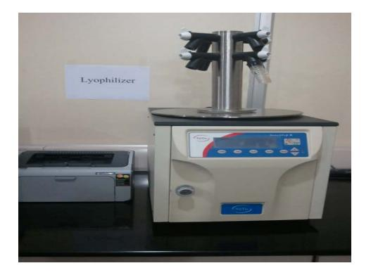
**Lyophilizer:** The Lyophilizer VirTis BenchTop have been designed to meet the needs of the most demanding research laboratories. Each system can be configured to meet your present and future needs. Condenser refrigeration packages of -55°C, -75°C, -85°C and -105°C can meet the demands of both aqueous or aqueous-solvent based formulations.
