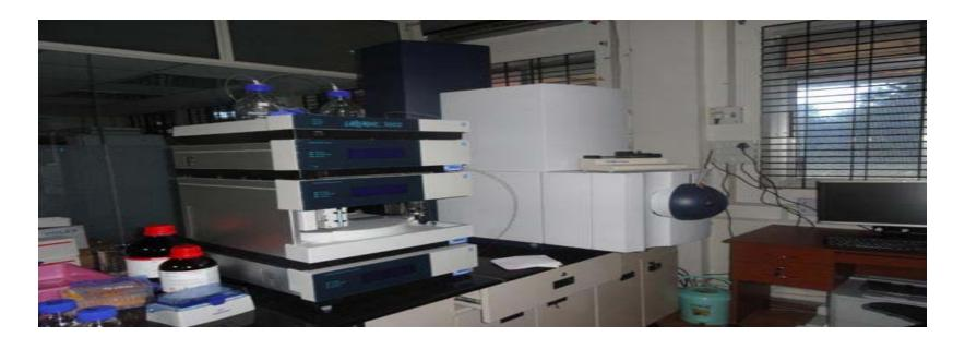
**Liquid Chromatography Mass Spectrometry (LC-MS):** Presently, SIC is equipped with Bruker Daltonik, Benchtop easy-to-use, High Performance Electrospray Ionization Quadrupole time-of-flight LC MS spectrometer designed for exact mass and true isotopic measurements. We analyse samples for other Schools within the Institute and from external commercial companies.
