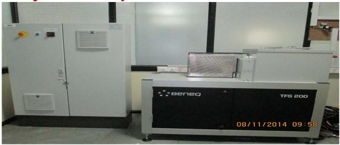
Atomic Layer Deposition (ALD): Equipment: TFS 200, BENEQ: Atomic Layer Deposition (ALD), as a thin film coating method, offers:
